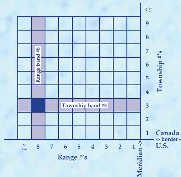
creasingly wide. This produced an offset between the townships along a line halfway between the baselines. The lines where these offsets occurred became known as correction lines.
